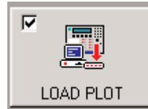
To load the wave form sampled by the 950B, simply (check the serial connection) press the key on the side ("LOAD PLOT"). The plot is thus loaded and displayed, and all the corresponding parameters read by the 950B (times and trigger levels) are updated on the screen. If you want to load the wave form present in the EEPROM memory in the 950B (permanently saved previously), it is first necessary to transfer it to the RAM of the 950B. This can be done
