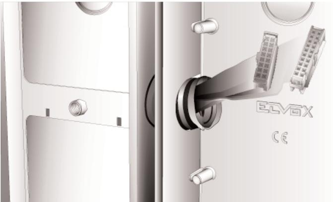
Fig. 7 - Example of installation of the flat cables on the back of the entrance panel with keypad and numerical display.
